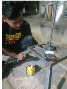
Figure 5. Current, Voltage and Electric Power (DC) Testing
