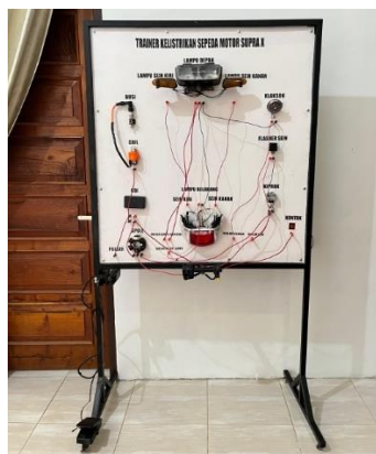
Figure 6. Supra X motorcycle electrical trainer
